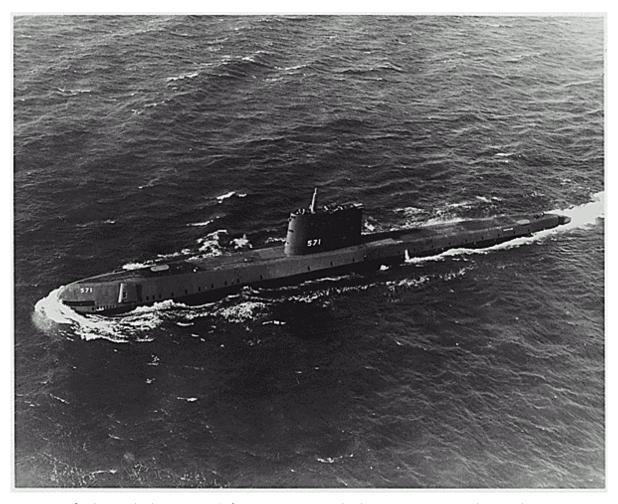
USS *Nautilus* (SS-571), the US Navy's first atomic powered submarine, on its initial sea trials, 20 January 1955.
