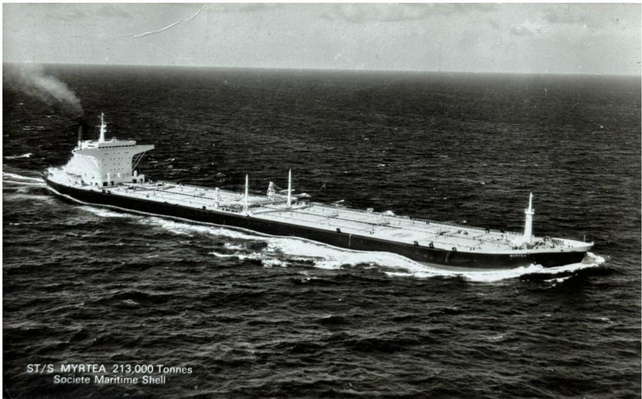
Photograph of the *Myrtea*. Being a “Very Large Crude Carrier” (VLCC), it was one of the first oil tankers above 200,000 tons deadweight—a measure of how much weight a ship can carry, as a sum of cargo, fuel, fresh water, ballast water, provisions, passengers, and crew—that began to dominate the world’s shipping lanes during the early 1970s.
