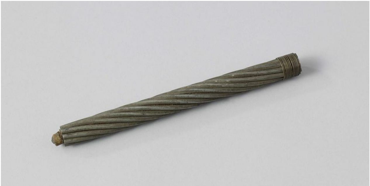
A section of telegraph cable, the copper wire protected by a layer of (probably) gutta-percha and paper, with steel on the outside, ca. 1865–1875.
