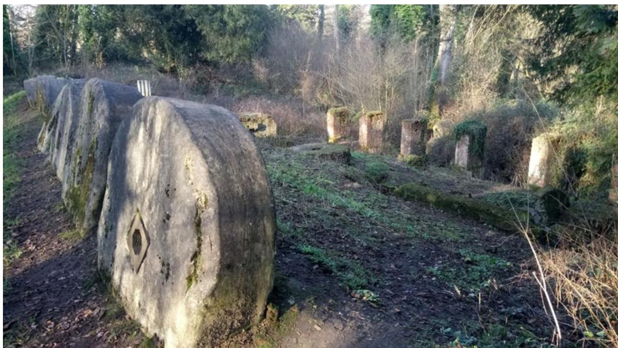
Walking eastwards through the site, one encounters these millstones ("edge runner stones"), which were stood on their sides to provide protection in the event of accidental blasts at a later stage of the site's development. Today, they are one of the works' most iconic features.
