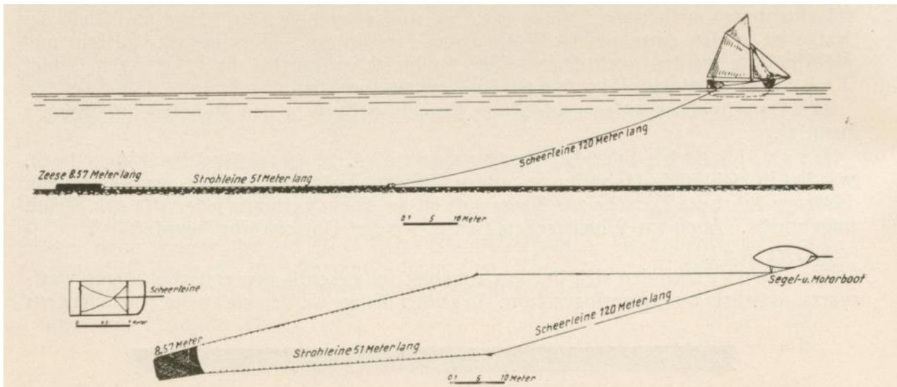
The otter trawl is a sack-shaped net, that is dragged over the ground by the fishing vessel to catch bottom-dwelling fish like flatfish.
