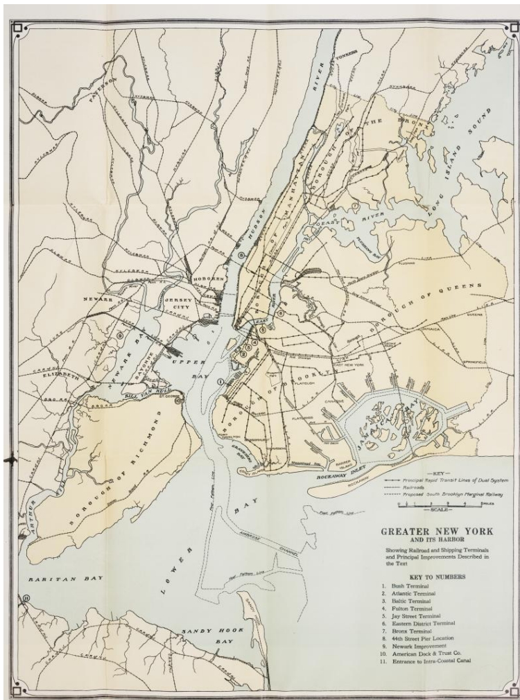
Fig. 1. Oceanic traffic leaving New York Harbor was fed by 12 railroads that either loaded freight cars on carfloats or offloaded material onto lighters or barges, a time- and labor-intensive process. More than nine thousand vessels traveled to the harbor each year making it one of the busiest, and without question, one of the most inefficient transportation hubs in the world. The combination of unprecedented weather and extreme wartime rail volume led to congestion and eventual gridlock.
