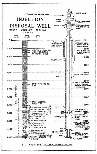
The 12,045-foot (3,671-meter) RMA injection disposal well was considered revolutionary for the time. In 1961, it was one of the deepest wells in the United States.
