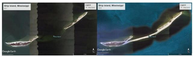
The aerial image at left shows Ship Island in 2017 before sand deposition and the aerial image at right shows Ship Island, Mississippi in 2019 after East and West Ship Islands were reconnected as part of the Mississippi Coastal Improvements Program.
