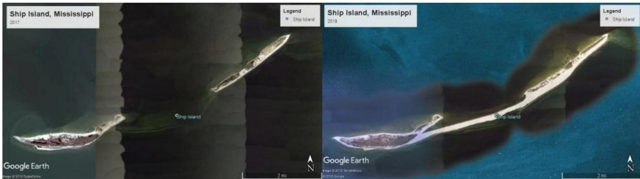
The aerial image at left shows Ship Island in 2017 before sand deposition and the aerial image at right shows Ship Island, Mississippi in 2019 after East and West Ship Islands were reconnected as part of the Mississippi Coastal Improvements Program.
