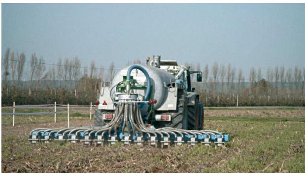
A slurry tank with an injection system.
