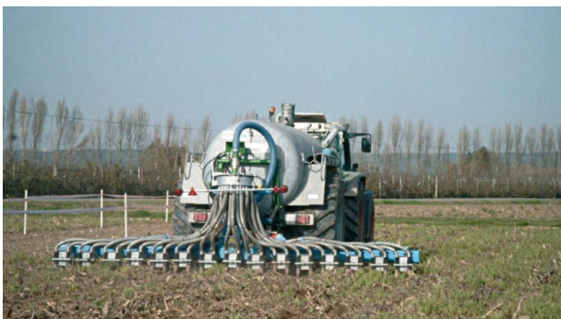
A slurry tank with an injection system.
