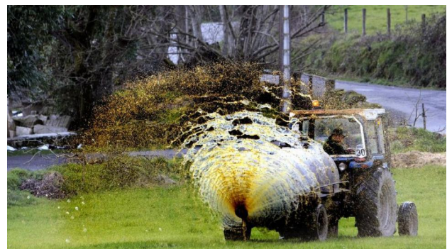
A slurry tank with a splash plate.
