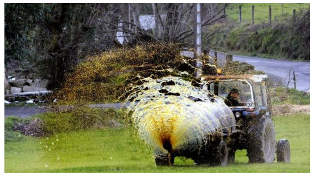
A slurry tank with a splash plate.
