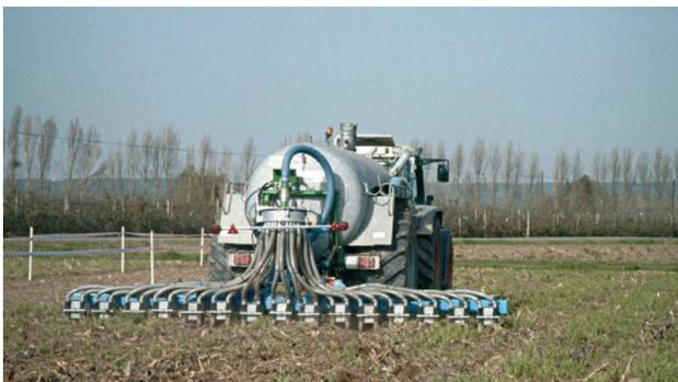
A slurry tank with an injection system.
