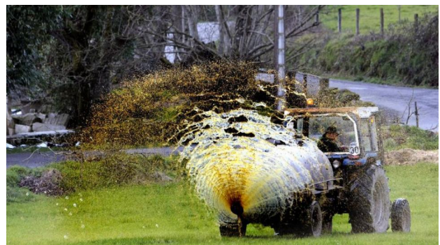
A slurry tank with a splash plate.
