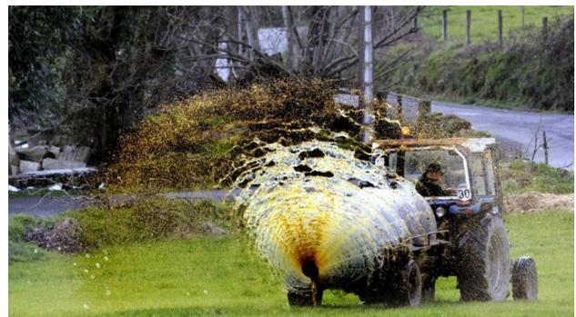
A slurry tank with a splash plate.
