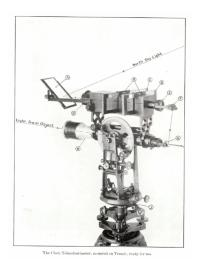
Fig. 2. Niagara Telecolorimeter.
