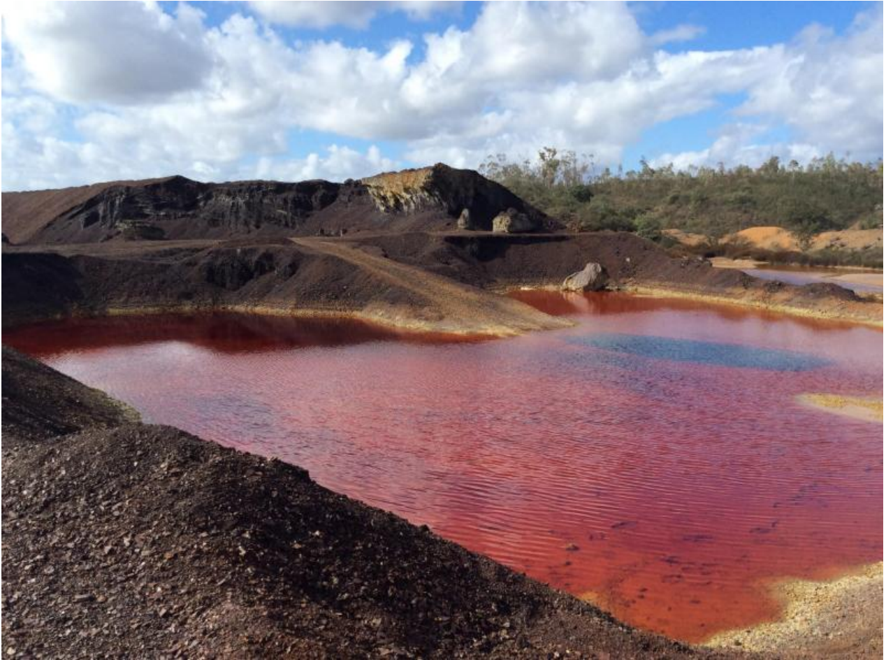
Remnant slag heap with acidic pond (pH ~2)
