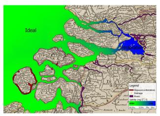
Reconstructed salinity of the Rhine/Meuse Delta and conditions of habitats for shipworms under drought conditions
