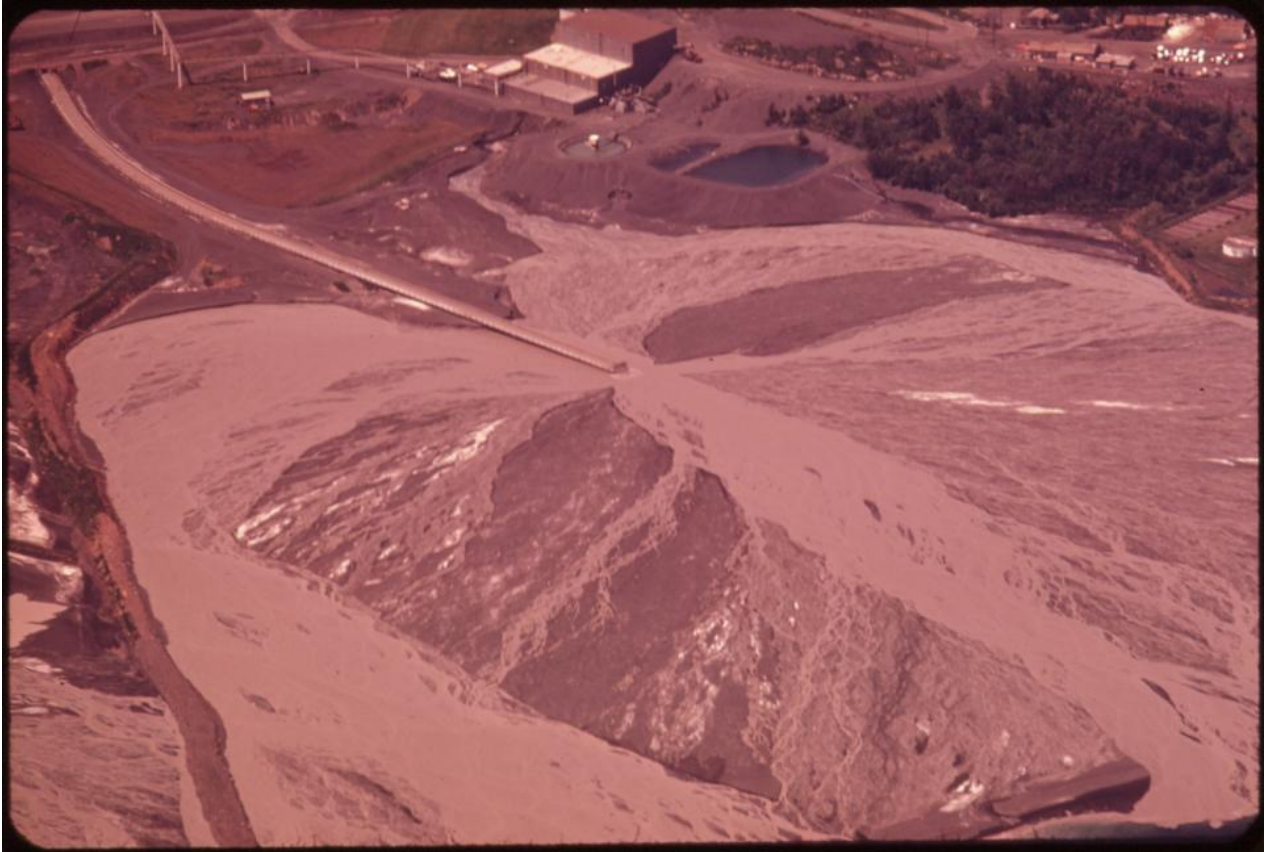
Taconite tailings from Reserve Mining Company are discharged via a chute into Lake Superior.
