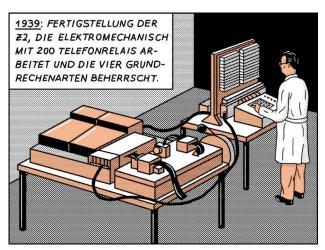
1939: Completion of the Z2. It functions with 200 electromagnetic relays and can perform basic arithmetic.
