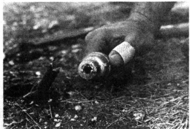
Note the "Seal" created in the end of the driver (the 1/4 inch nipple screwed into one of the reducers).
